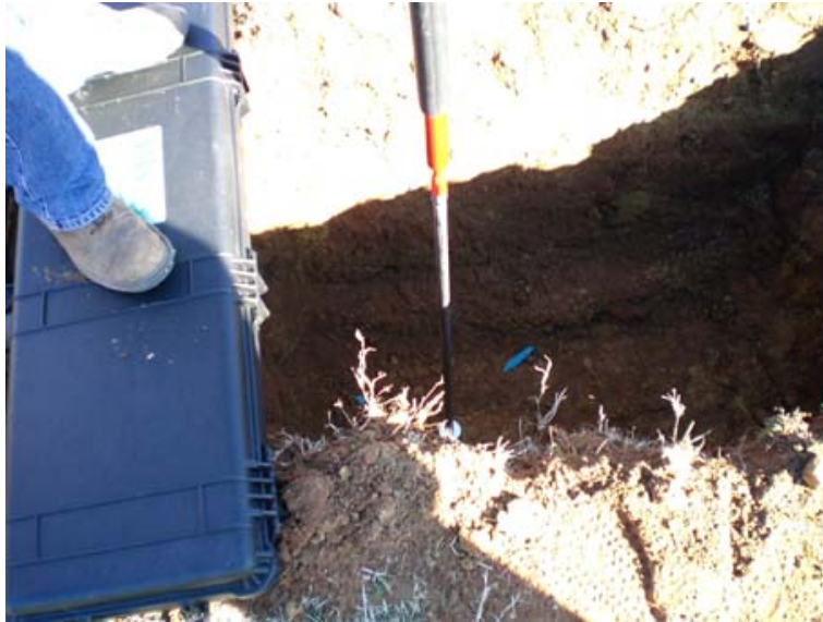
Photo No. 3: B-1 boring soil sampling in the bottom of the former grave.
