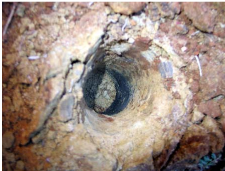
Photo No. 8: Close-up view of soil boring B-2 in the grave site of the subject. The lower dark zone (approx. 1-2 inches) is due to friction between the soil coring device and the sandstone and represents the top of bedrock. No indication of organic material.
