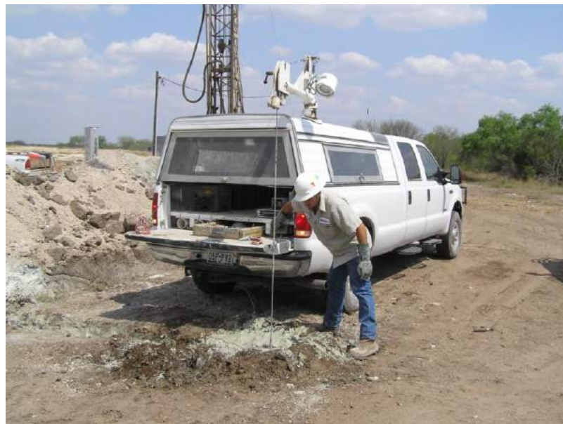
Figure 25 – Geophysical Well Logging Activities along the Primary Ore Zone (from MULLC)
