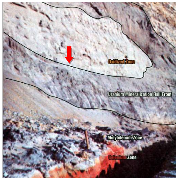
Figure 13 – Typical Uranium Occurrence in Wall of Open Pit in South Texas of 1970s. (after Dickinson and Duval, 1977)
