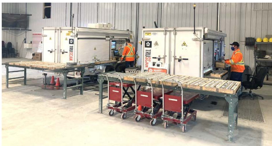
Fig. 1. In-field, trailer-based X-ray fluorescence scanning units operating in the core shed at Red Chris, British Columbia.
