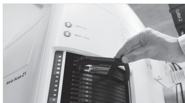
Figure 2 Tray magazine of ZEISS Axio Scan.Z1
