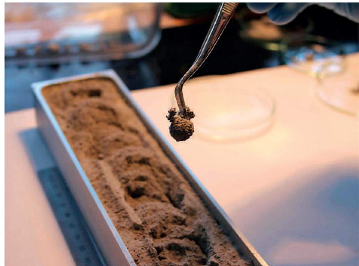
Fig. 13: A small sample was successfully printed in a vacuum by injecting the binder underneath the regolith surface.
