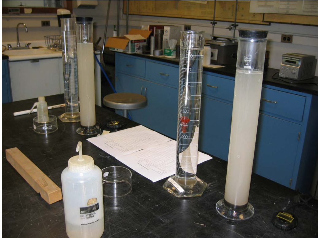
Figure 3.4 Hydrometer test in progress for fine particles
