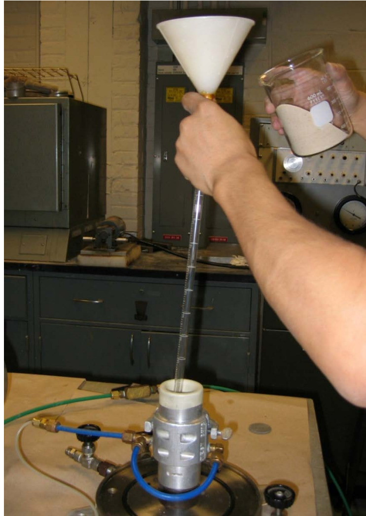
Figure 3.12 Using a funnel slowly pour the soil into the mold
