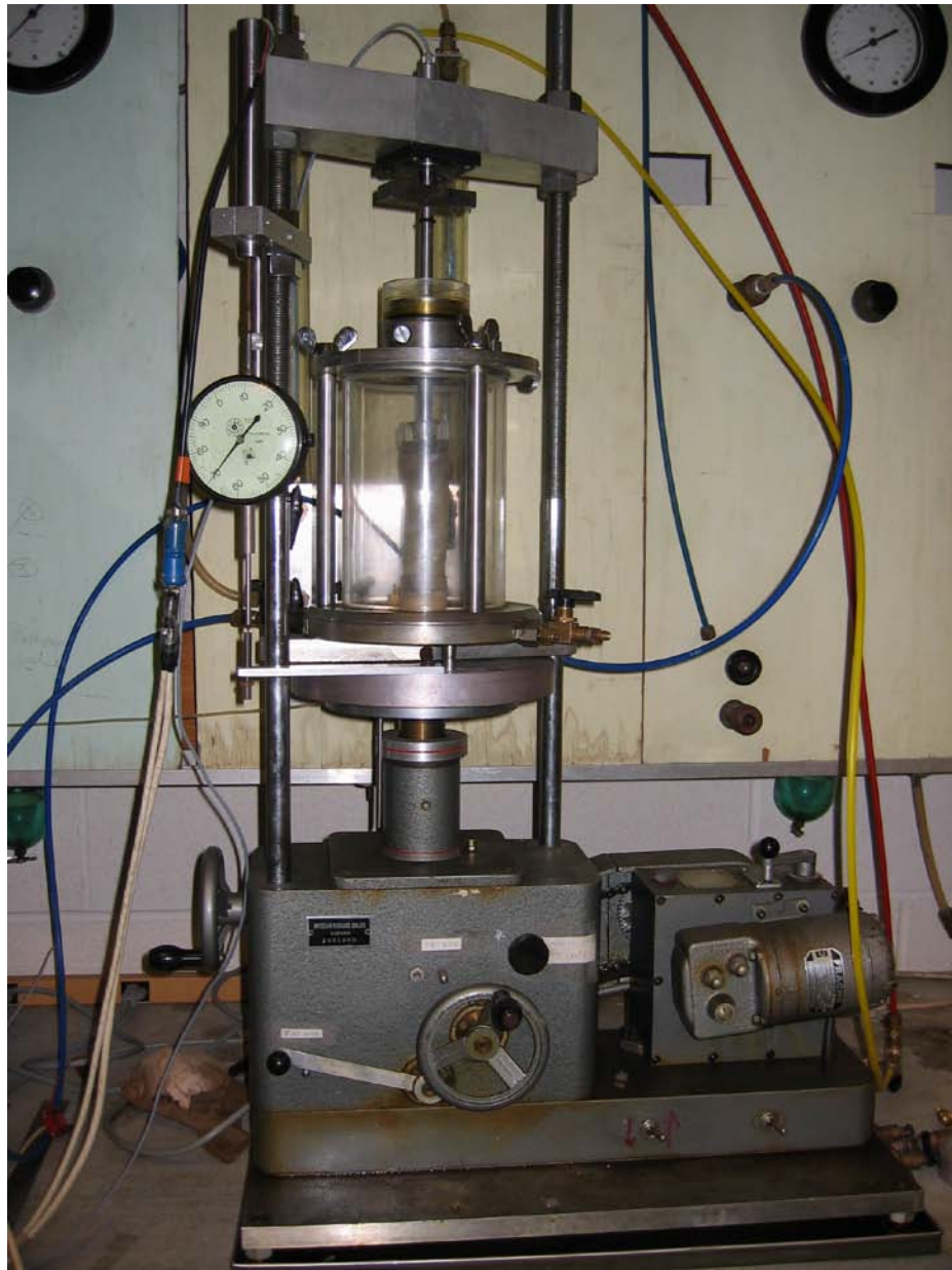
Figure 3.14 Triaxial cell on the load frame connected with LVDT
