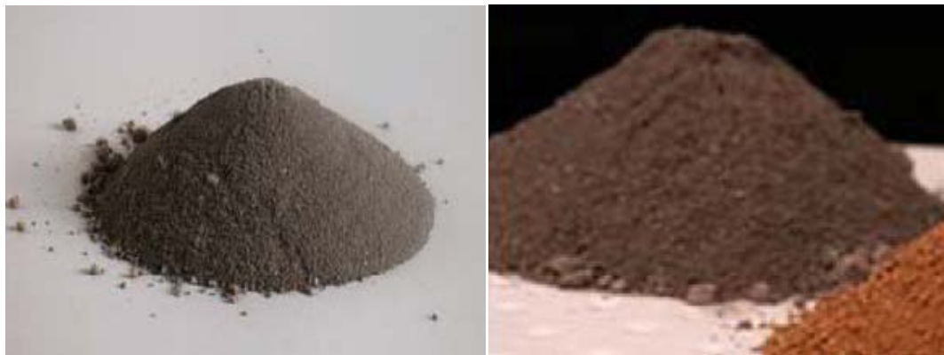
Figure 3.2 JSC-1AF (left) and JSC-1A (right)
