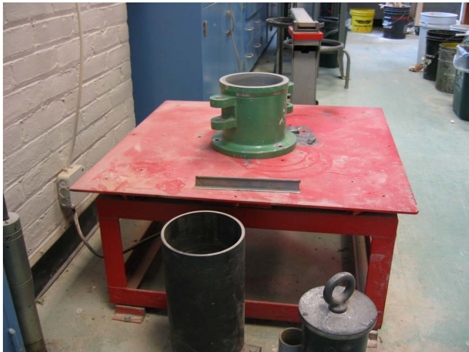
Figure 3.9 Compaction mold bolted on shake table
