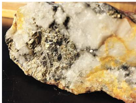
Figure 8B – Quartz Vein with Euhedral and Anhedral Pyrite and Pyrrhotite (magnetic) (From Vai Dao Mine Dump) Click on Figure to Enlarge
