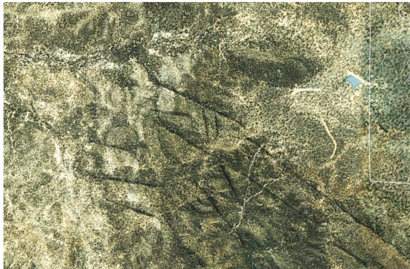
Figure 21 - Joints and Faulting at the Northern Terminus of the Magnetic Anomaly. (After Google Map – Lineaments Emphasized)
