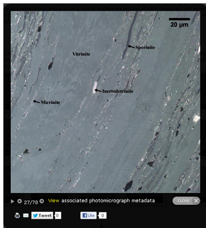
Fig. 2. Screen capture image of the gallery viewer window displaying a photomicrograph taken in incident white light under oil immersion.
