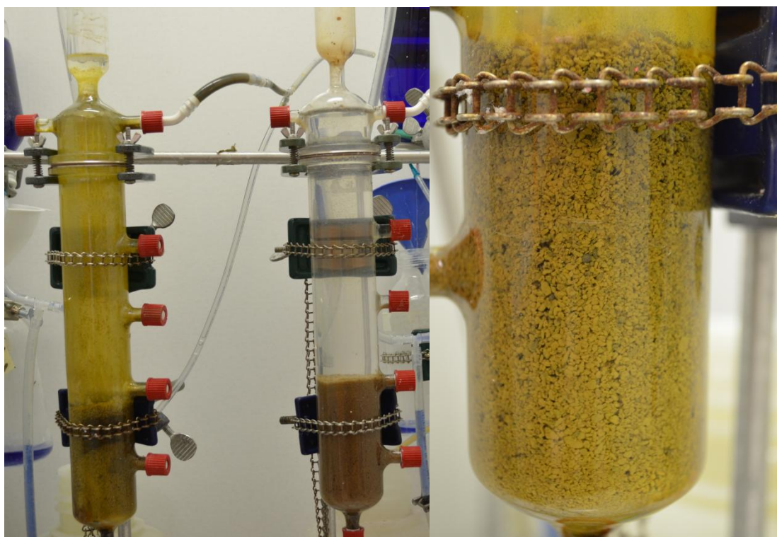
Fig. C.3. Evidence of mineral precipitation. The picture was taken 70 d after the addition of \text{As}^{\text{V}} . A yellow precipitate is clearly present in reactor 1 (left), in the liquid medium and on top of the sludge. No precipitate is observed in reactor 2 (right), where the medium appears clear and the sludge clean.
