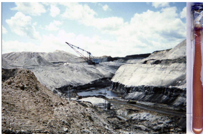
Fig. 9. View of Pavlovka coal deposit, Russian Far East and pure REE + Y oxides extracted from the high-REE + Y coal ash (0.4% REY 2 O 3 ) of the deposit (test-tube is 100 mm long).
