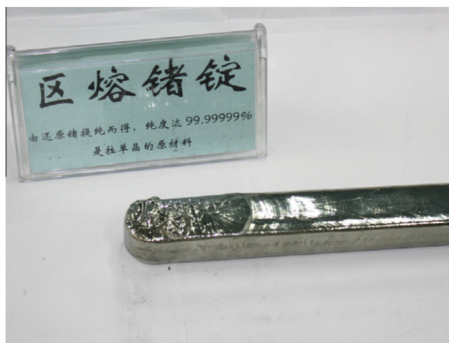
Fig. 2. High-pure metallic germanium (99.99999%), produced by Xilinguol Tongli Ge Refinery Co., Ltd. from Ge-bearing coal of the Wulantuga deposit.
