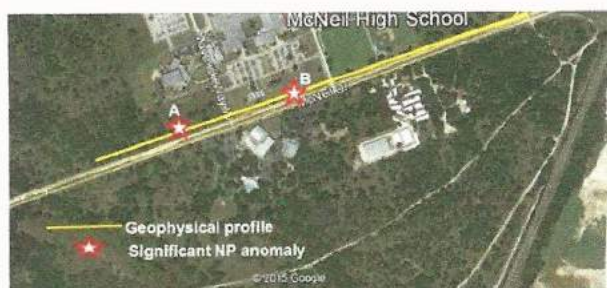
Figure 10. Location of a geophysical profile—a mile long—along the McNeill Road and McNeil High School in north Austin, Texas. Two stars shown with red and white colors (A and B) are locations where significant NP anomalies are observed.
