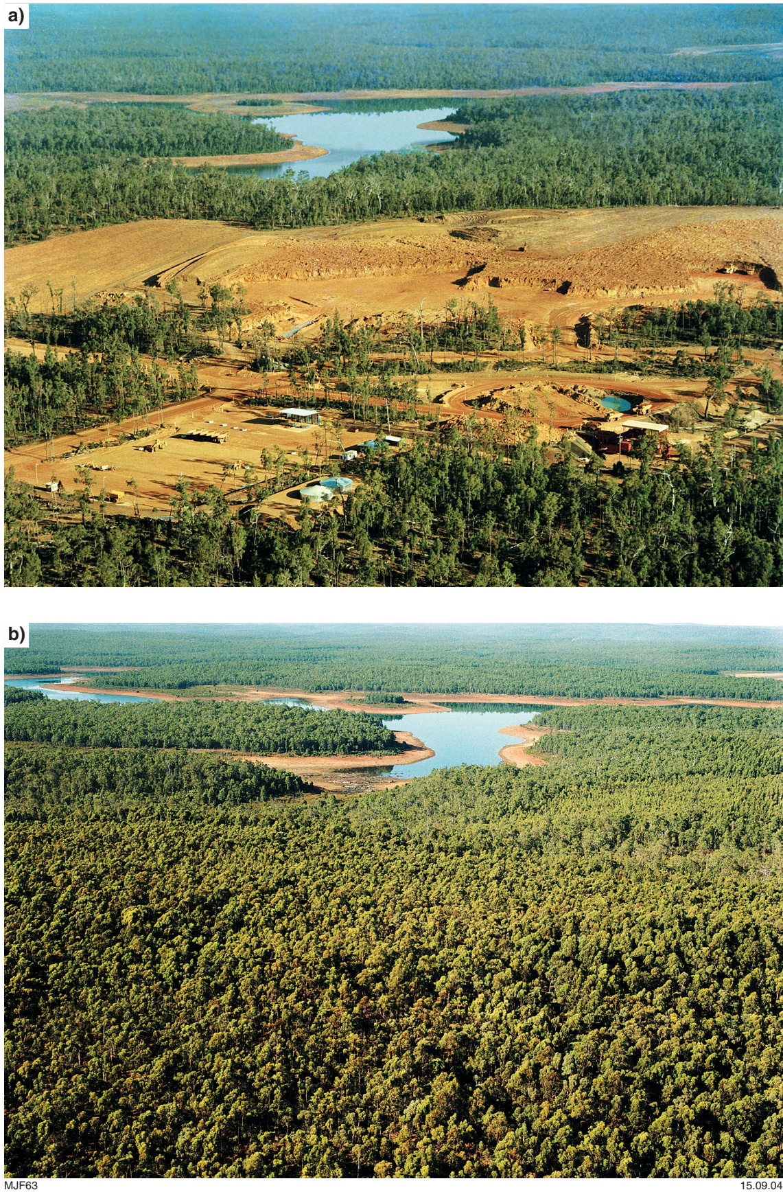
Figure 10. Photographs of mining area at Huntly: a) mobile crushing plant and other mine infrastructure in front of cleared partially mined area, with North Dandalup reservoir beyond; b) same site four years later following rehabilitation of all the cleared areas and restoration of the landforms (photos courtesy of Alcoa World Alumina Australia)
