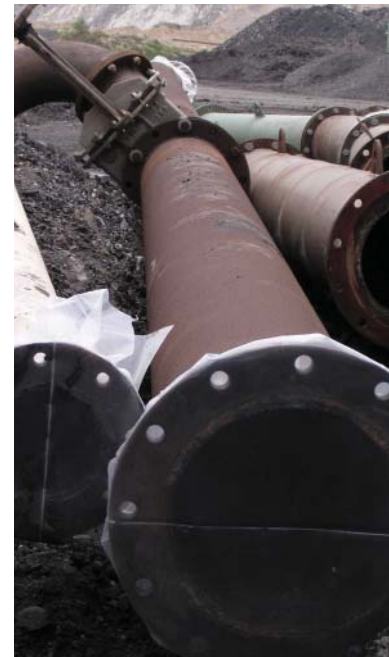
NORM contaminated pipes from a coal washery
