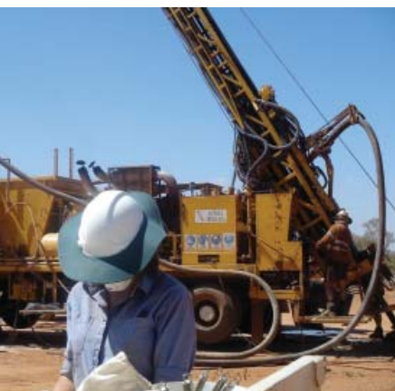
Reverse Circulation drilling Nolans Bore
