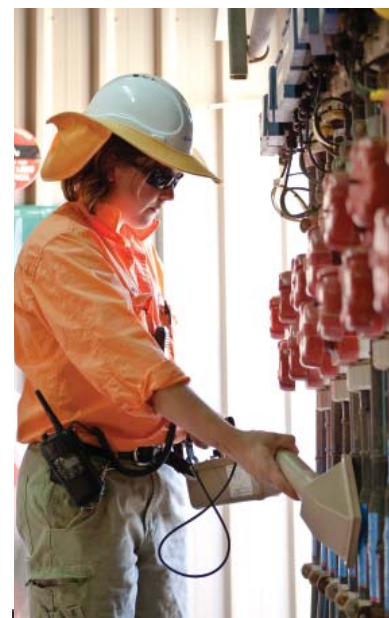
Surface contamination check in Well House Long lived alpha filter count Beverley
