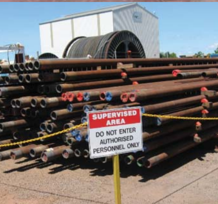
NORM contaminated tubing from oil production wells
