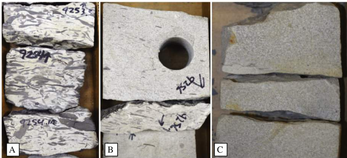
Fig. 9. Representative core samples showing characteristics of facies association 1 – fluvial distributary channels (each core sample is 5 cm wide except in C which is 9 cm wide; see well log in Fig. 4) A. very fine-grained sandstone with carbonaceous detritus and carbonized wood fragments. Rip-up clasts of plants debris and elongate mud chips show a crude alignment. Pieces of wood several centimeters in length are locally abundant. B. Sandstone with mud chips scattered throughout and organic debris as laminae. Plant fragments occur locally on bedding planes. There is no evidence of burrowing. C. Very fine-grained structureless sandstone.
