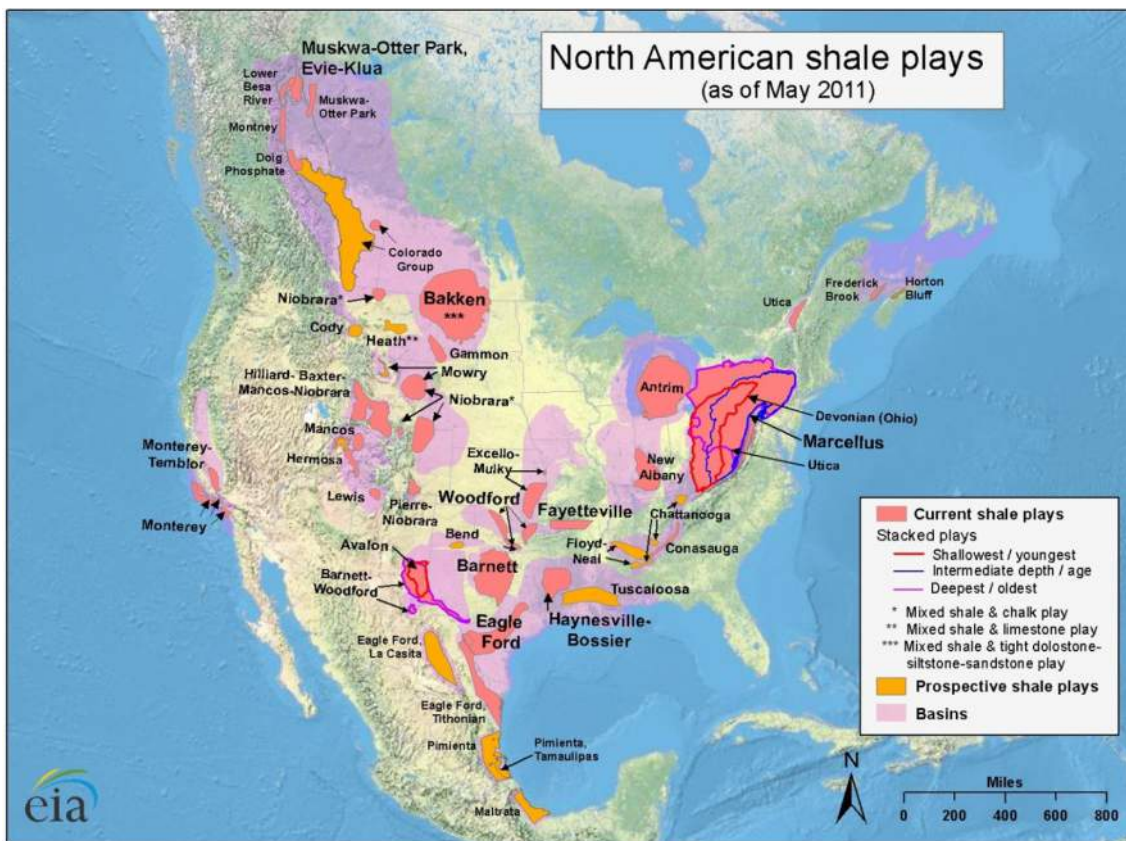
Figure 18. Locations of shale and tight oil plays in North America. From EIA (2011).
