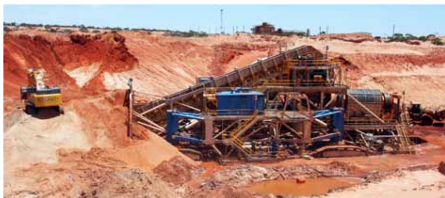
Figure 2 Sand containing HM is pushed by dozer to the mining unit plant located within the pit. (Photo 407878)
