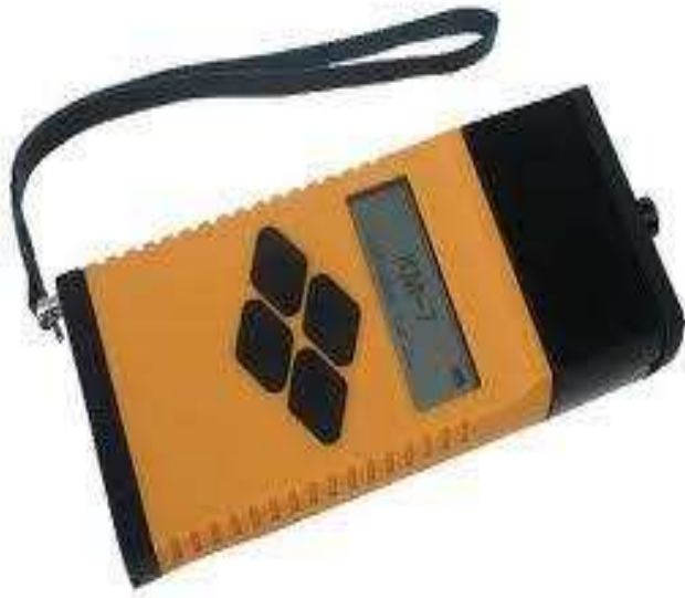
FIGURE 16: PICTURE SHOWING A POCKET SIZE KM-7 MAGNETIC SUSCEPTIBILITY METER.
