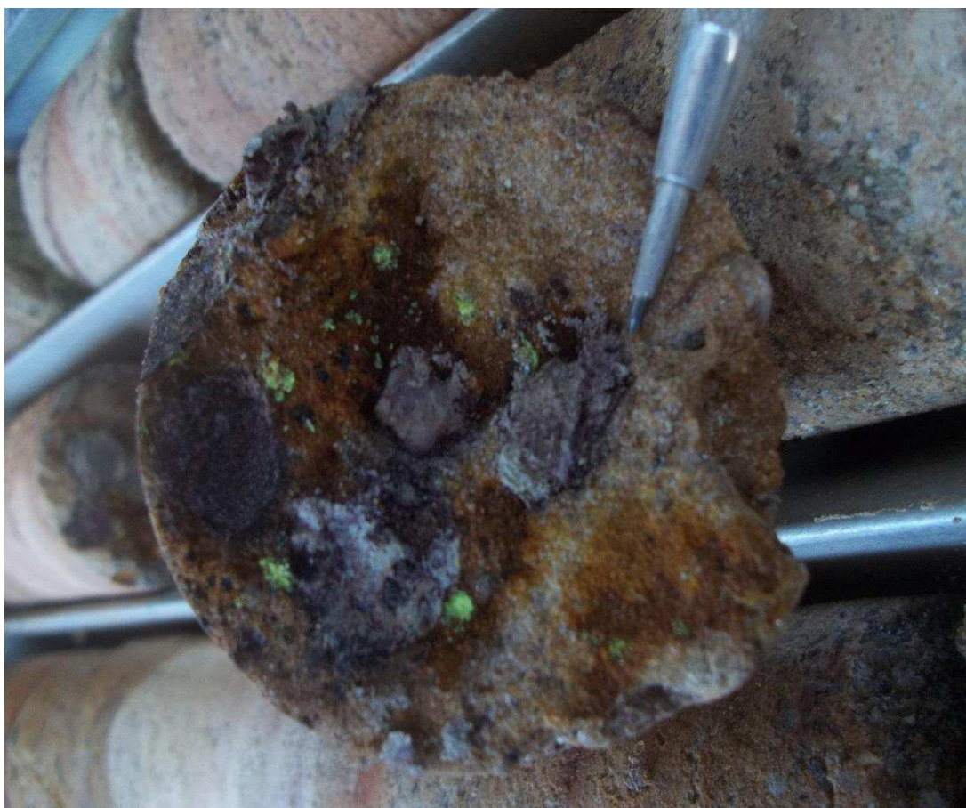
FIGURE 10 PICTURE SHOWING DISSEMINATED URANIUM MINERALIZATION IN A SANDSTONE. MINERALS ARE SEEN AS BRIGHT GREENISH YELLOW.
