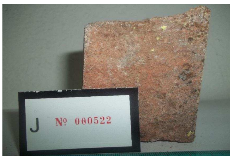
FIGURE 22: PHOTOGRAPH COARSE TO MEDIUM GRAINED SANDSTONE SHOWING TRACES OF URANIUM MINERALIZATION SHOWN AS BRIGHT GREEN-YELLOW MINERALS.
