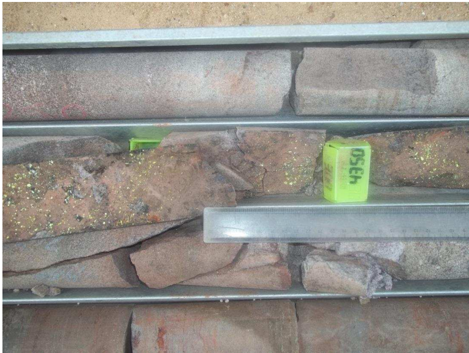
FIGURE 12 PICTURE SHOWING MINERALIZATION IN WHAT WAS FRACTURE ZONE.
