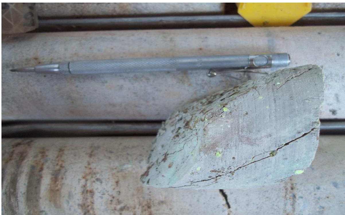
FIGURE 11 PICTURE SHOWING URANIUM MINERALIZATION IN MUDSTONES.
