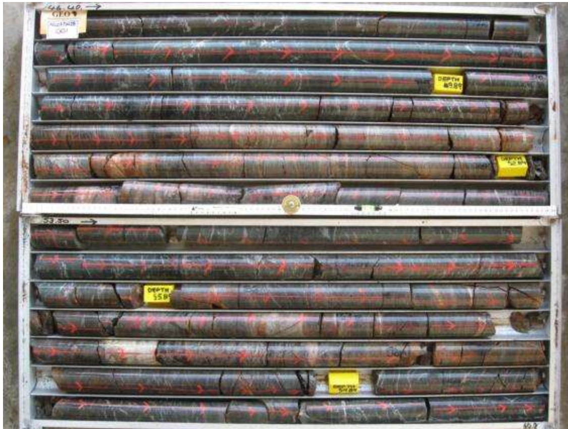
Plate 13.3 Drill core from Hole NBLOFDH2B001 showing high quality of core recovery with meterage marking and orientation
