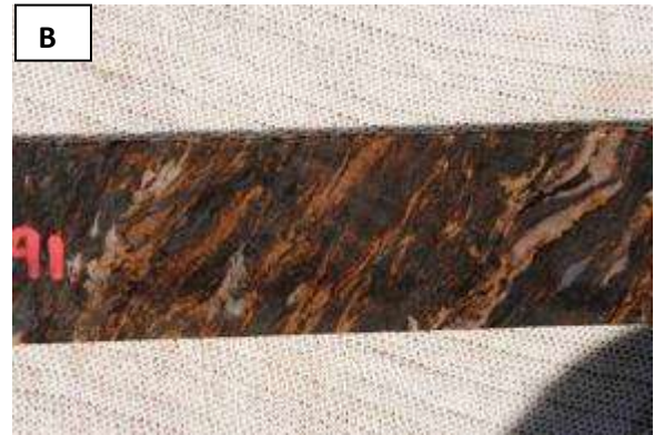
Plate 13.5 A – white to grey massive albitite, fractured and veined by white calcite, and later by brown carbonate. B - shear zone infused with brown carbonate and green phlogopite. Core width is 5 cm.
