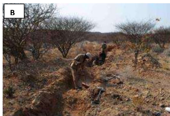
Plate 12.2 A – digging trenches on Area 2B with a backhoe. B- cleaning trenches in preparation for sampling and mapping.
