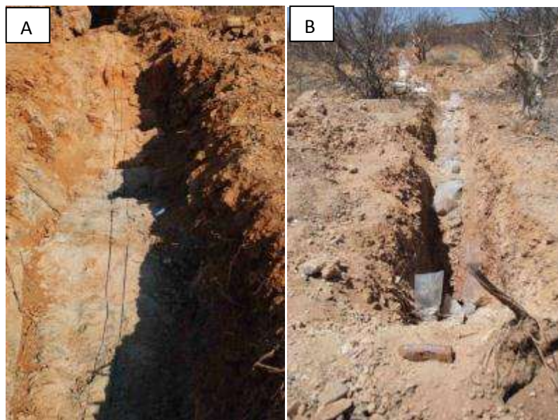
Plate 14.1 A - trench floor cut by diamond saw and ready for sampling. B - bagged samples in trench floor ready for collection
