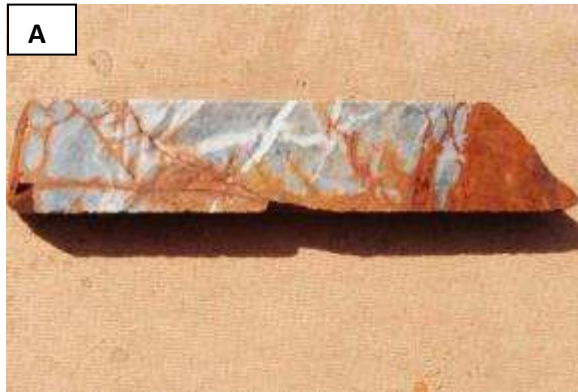
Plate 13.5 A – white to grey massive albitite, fractured and veined by white calcite, and later by brown carbonate. B - shear zone infused with brown carbonate and green phlogopite. Core width is 5 cm.
