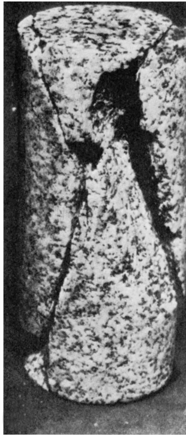
Fig. 3. Failure of cylindrical rock test specimen, combined cataclasis and cleavage, granite. (After Hawkes & Mellor 1970)
