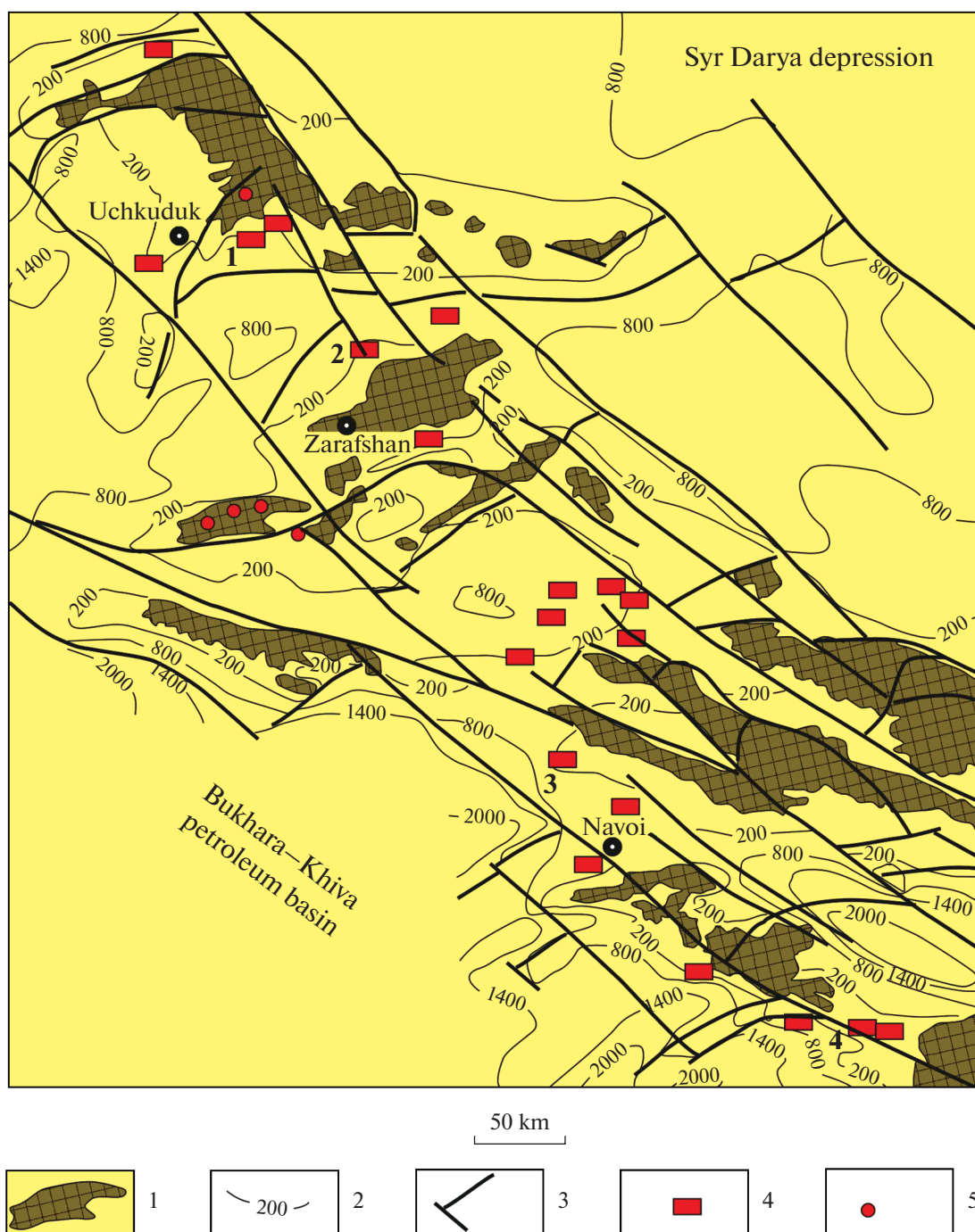
Fig. 4. Kyzylkum uranium ore province (from Geological-economic ... , 2008, with simplifications). (1) Paleozoic basement highs from under sedimentary cover; (2) depth of basement roof (m); (3) faults; (4) deposits (numbers: (1) Uchkuduk; (2) Sugraly; (3) South Bukinay; (4) Sabyrsay); (5) ore occurrence.
