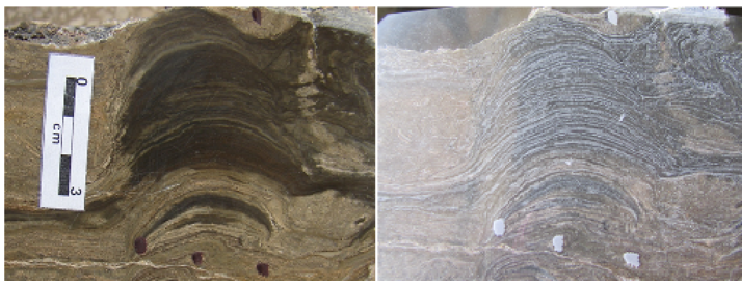
Fig 10. Stromatolite within impure dolostone and corresponding CN film showing dense alpha tracks.
