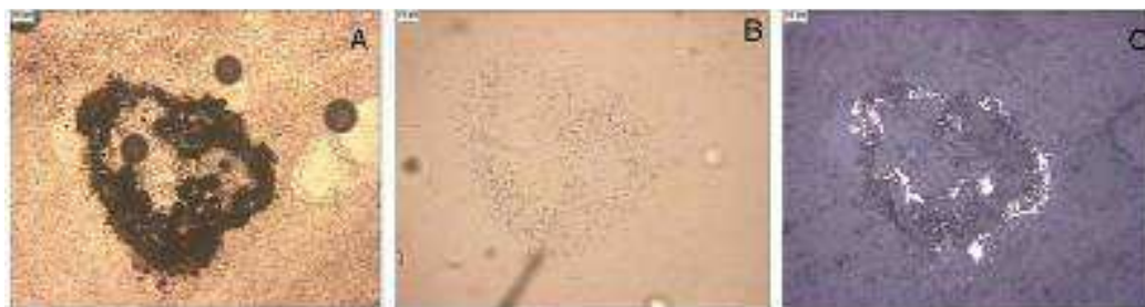
Fig 8. A. Framboidal pyrite as aggregates in association with peloids and carbonaceous matter (20x, TL, 1N). B. Sparse tracks due to adsorbed uranium on carbonaceous matter (20x, TL, 1N). C. Peloid with pyrite and carbonaceous matter (20x, RL, 1N).
