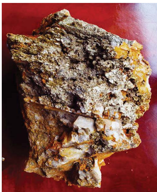
Figure 11: Gold-Sulfide (Pyrite and Pyrrhotite) in Quartz Breccia of Fault Zone in Pit and Stockworks (in Lang Sen area), mostly oxidized.
