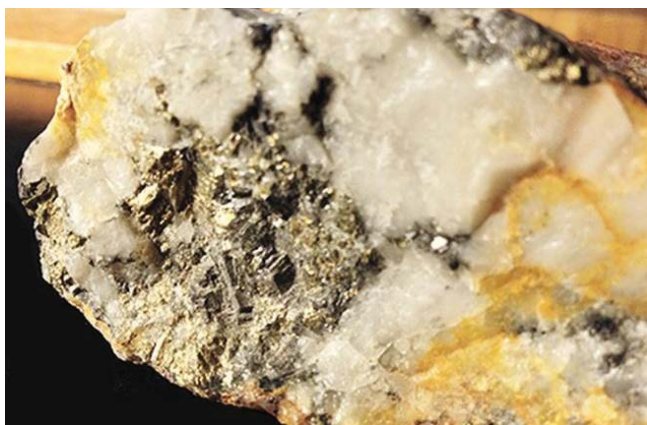
Figure 10: Quartz Vein with Euhedral and Anhedral Pyrite (From Vai Dao Mine Dump).
