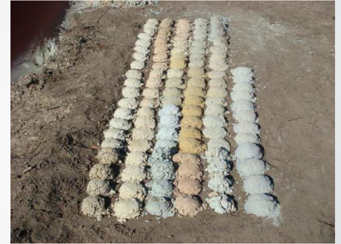
5 Ft-Drilling Samples down to 560 Feet Note: Oxidized (orange) and Unoxidized or Reduced Samples (Gray).
