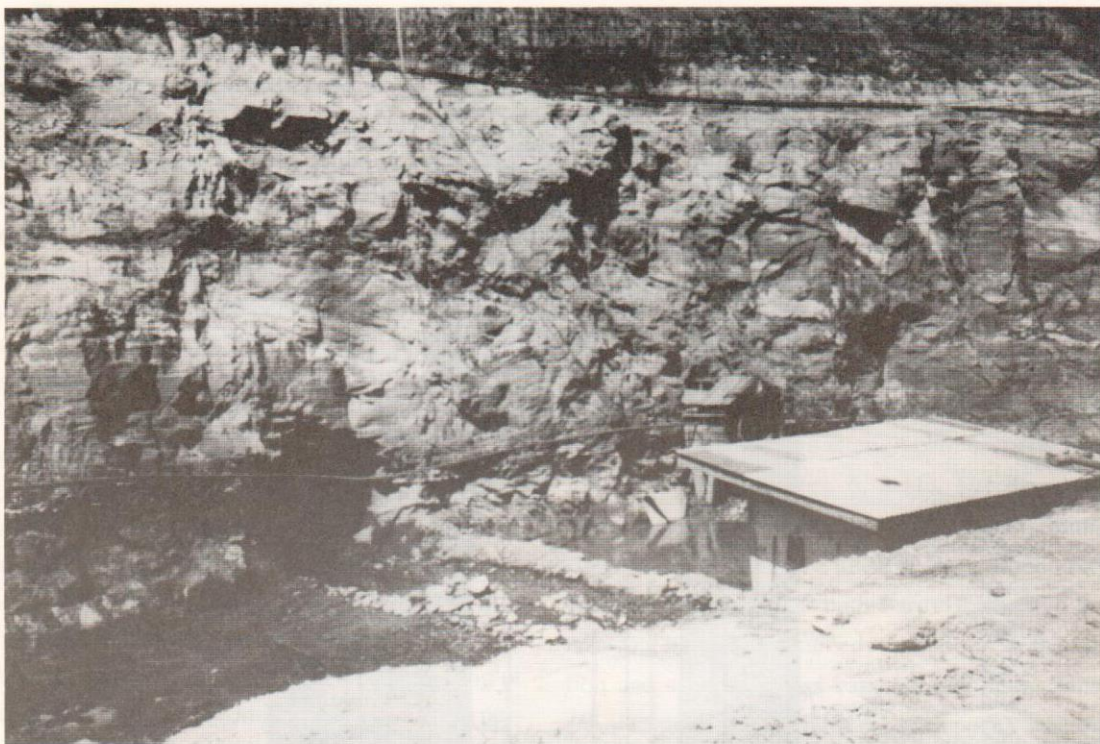
Fig. 7 — Deltaic progradation over lagoonal sediments (silt and coal). Growth-faults are enhanced by silt injection. Open-pit Figueira Mine, State of Paraná.
