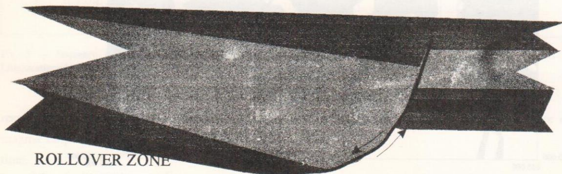
Fig. 5 — Basic geometry and main attributes of a growth-fault affecting the coal section. Main attributes: 1 — Listric Fault plane with no throw in the lower and upper ends of the fault trace. 2 — Beds dip against the fault plane in the downthrown block. 3 — Sandstones thicken in the downthrown block and thin towards the rollover zone. 4 — Sliding surfaces produced in coal or in associated shale and siltstones
