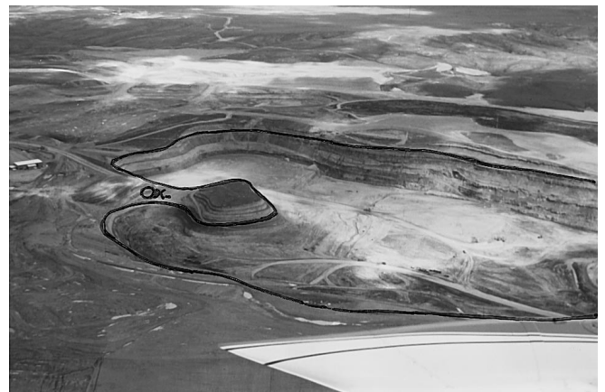
Figure 4 Aerial view of Highland Mine, southern Powder River Basin, Wyoming. The horseshoe-shaped pit outlines a plan view of an ore roll, with an oxidation tongue extending into it from the left
