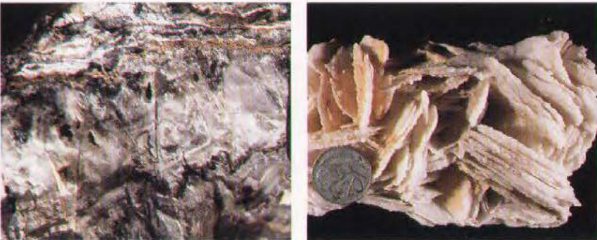
Fig. 4.2 (L.) Banded botryoidal quartz vein from the Sleeper LS deposit, Nevada [44]; note electrum bands and quartz after bladed calcite (photo by J. Saunders). (R.) Coarse bladed calcite from the Martha Hill LS deposit, New Zealand (photo by S. Simmons).
