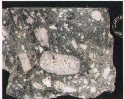
Fig. 4.4 Diagnostic textures of HS epithermal deposits. (L.) Vuggy quartz caused by leaching of sanidine phenocrysts (≤4 cm long) by acidic fluid (pH <2 [55]). (R.) Same rock (quartz latite porphyry) altered to alunite-kaolinite in the alteration halo to vuggy quartz ore zone of Summitville deposit.
