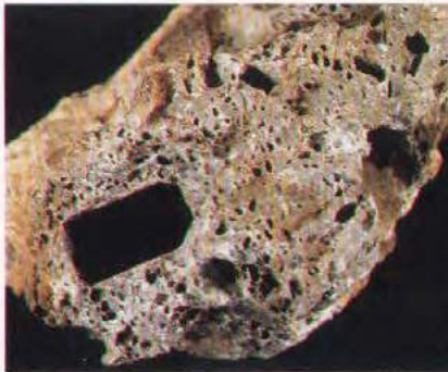
Fig. 4.4 Diagnostic textures of HS epithermal deposits. (L.) Vuggy quartz caused by leaching of sanidine phenocrysts (≤4 cm long) by acidic fluid (pH <2 [55]). (R.) Same rock (quartz latite porphyry) altered to alunite-kaolinite in the alteration halo to vuggy quartz ore zone of Summitville deposit.
