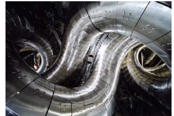
The Superconductor Coils Inside the LHD Vacuum Chamber
