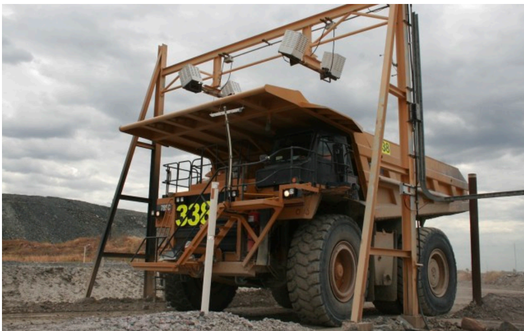
Mine truck carries rock under the discriminator which measures the radioactivity level to determine if the material is ore or waste.
