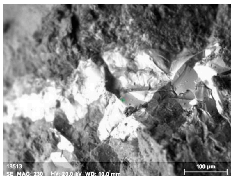
Figure 13. Mineral phase of thorianite shown as a streak in orthite.
