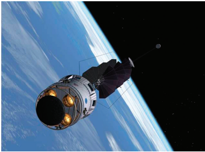
FIGURE 9. Illustration of tethered gravity generation via rotation around a common center of gravity using a counterweight (courtesy of National Aeronautics and Space Administration Archives). v = rotational velocity; \Omega = angular momentum of the combined unit; R = radius of the combined unit.
