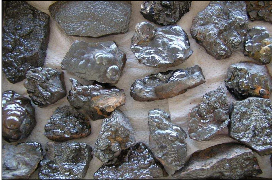
Figure 7.2 Botryoidal structure in goethite. Morocco.
