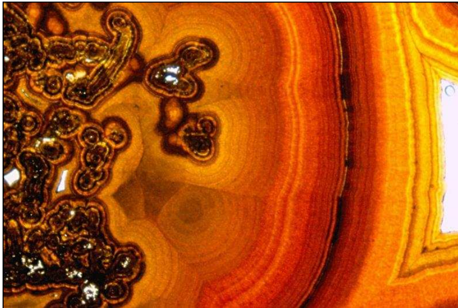
Figure 7.5 Colloform and banded texture in wood tin, with interlayers of hematite (black). Black Range, New Mexico. Transmitted light.
