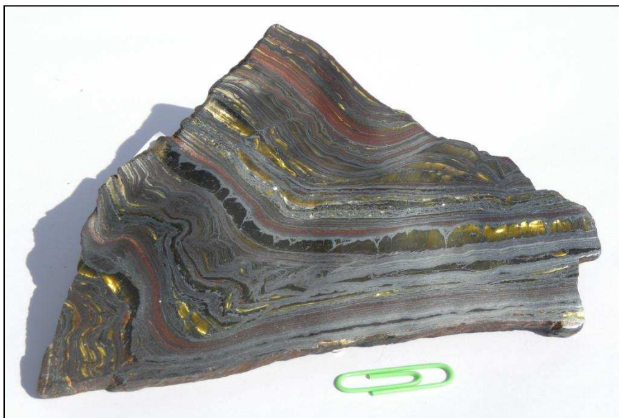
Figure 7.66 Archean Banded Iron Formation (BIF), consisting of hematite (gray), jasper (red), and tiger eye (yellow, silicified crocidolite or blue asbestos). Ord Ranges, Western Australia, about 1,000 miles north of Perth.
