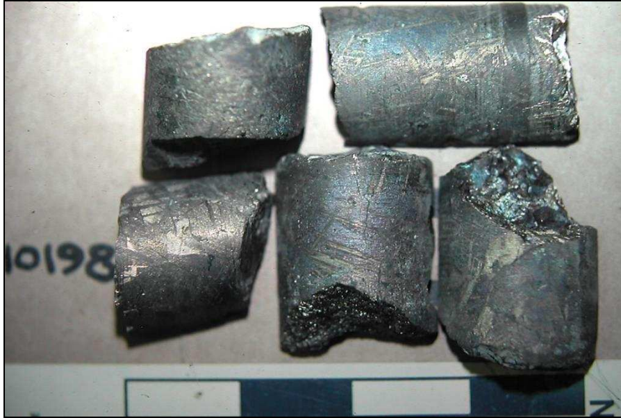
Figure 9.44 Tarnished talnakhite in core from Local Boy ore zone, Mesaba deposit, Duluth Complex. Photo courtesy of Mark Severson, NRRI, University of Minnesota, Duluth.
