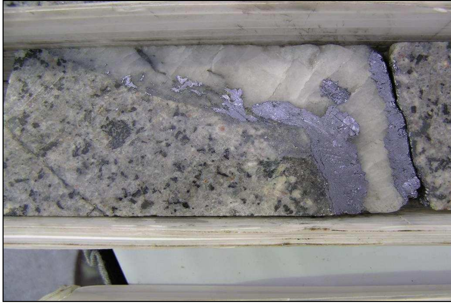
Figure 9.28 Molybdenite (bluish gray) in quartz vein, Leon deposit, Canada.
