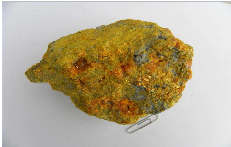
Figure 9.30 Orpiment (yellow) and realgar (red) from the Carlin Trend, Nevada. Specimen courtesy of Al Hofstra, USGS.
