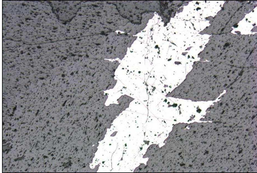
Figure 7.15 Silver-bearing tetrahedrite veinlet in siderite, Crescent mine, Coeur d' Alene district, Idaho. Note selective replacement of carbonate by tetrahedrite, guided by rhombohedral cleavage. 5x.
