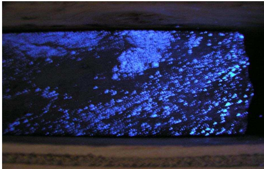
Figure 7.79 Scheelite in core under the black light. Cantung skarn deposit, Cantung, Canada.
