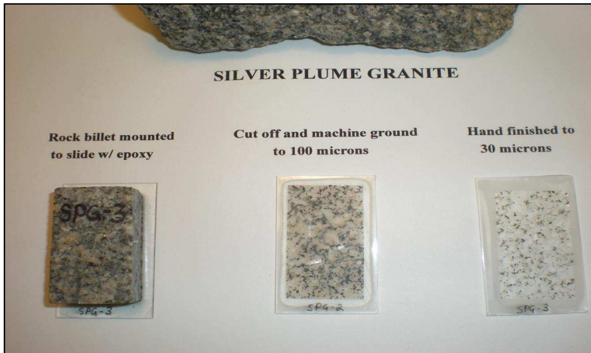
Figure 3.1 Three steps in the preparation of a polished thin section 30 microns in thickness.
