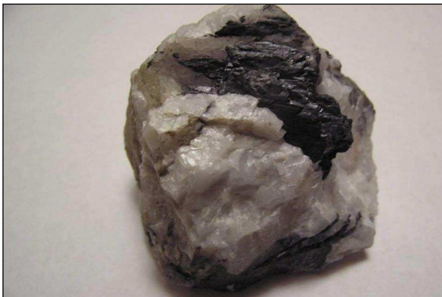
Figure 7.81 Wolframite in quartz, Hunan province, China. Specimen courtesy of Jim Elliott, USGS retired.
