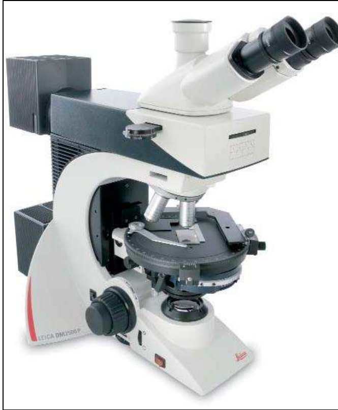
Figure 2.5 Leica petrographic microscope, Model DM2500P, equipped with both transmitted and reflected light capabilities.
