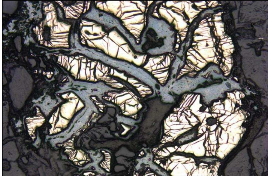
Figure 9.15 Supergene chalcocite (blue) replacement of pyrite. Santa Rita, NM.
