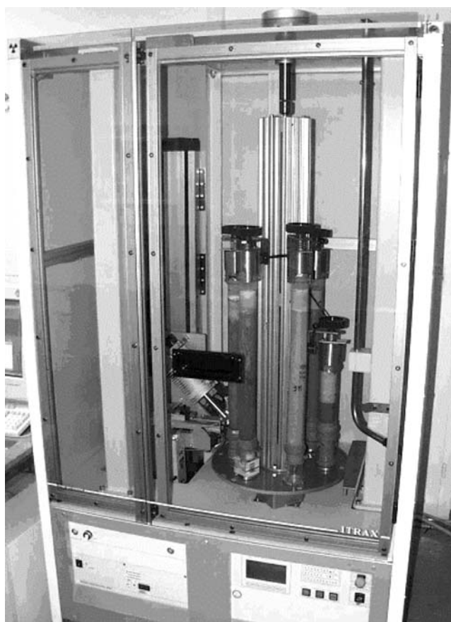
Fig. 7.127. XRGs equipped with columns
