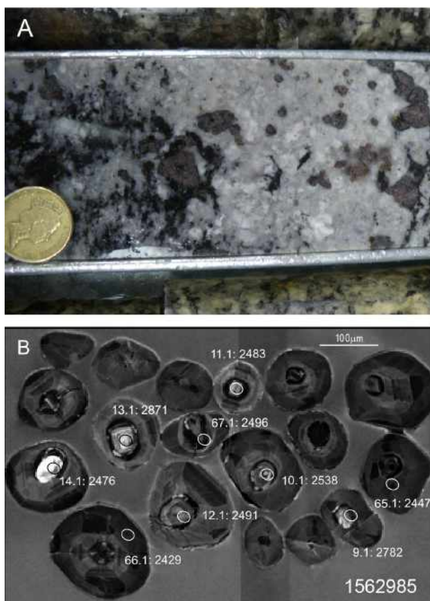
Figure 28. a) Photograph of core from CD-1, sample R1562985. (Photo 413528) b) Representative cathodoluminescence image of zircons from sample R1562985 showing the difference in age between metasedimentary cores and metamorphic rims.
