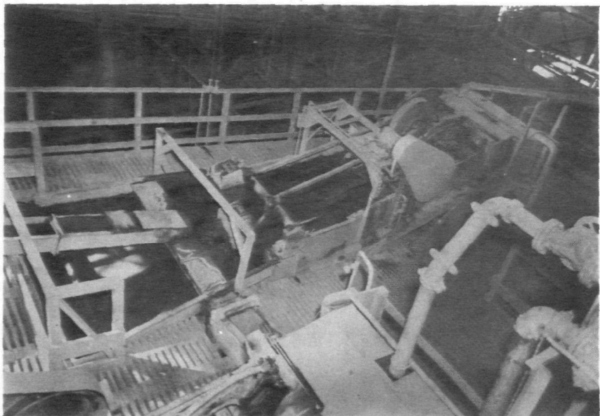
The solids are removed from the leached ore slurry in classifiers. A rake classifier is shown. (Photograph courtesy of The Anaconda Company)
