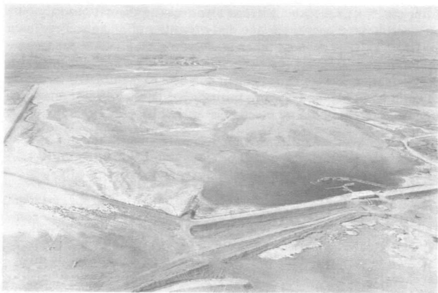
One of the industry's most extensive tailings pond areas is shown above. In this case liquid is decanted from the pond and injected into a deep well for ultimate disposal. (Photograph courtesy of The Anaconda Company)
