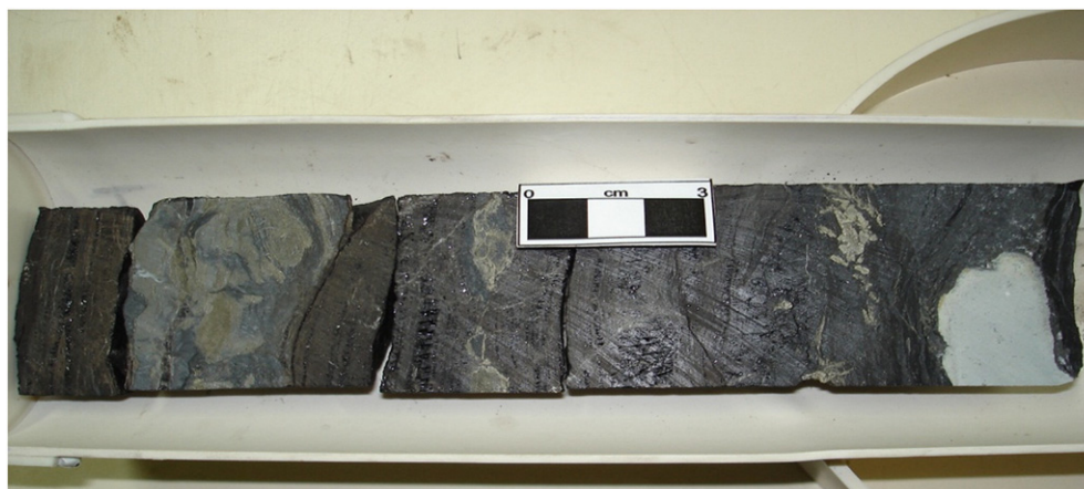
Fig. 6. Example of core samples used for a research on organic facies and organic maturity profiles (from Mendonça Filho et al., 2011b).
