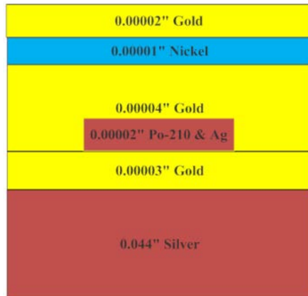
Figure 38. Typical design of a Po-210 alpha source. The polonium 210 foil is made of 10% polonium and 90% silver
